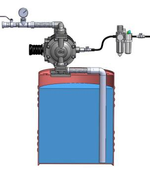
The diaphragm pumps are able to transfer fluids at 6 meter of deepness. Cavitation might obstruct the operation. To prevent this, the air in the hose between the pump and fluid should be discharged.
