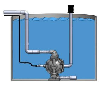
Diaphragm pumps can also be used as submerged pump. It is necessary to maintain the exhaust port of the pump above the liquid surface with pipe or hose.
