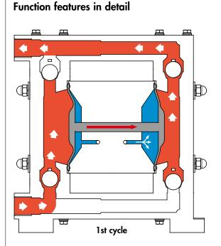
FLUX air-operated diaphragm pumps are positive displacement pumps consisting of two pump housings and one control valve part. Diaphragms within the pump housings securely separate the liquid section (red) from the air section (blue). Both diaphragms are connected by a selector shaft which is located in the control valve part.
