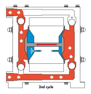
Compressed air inflating alternately the air sections causes a movement of the diaphragms (1st and 2nd cycle). The subsequent transfer operation is controlled by a control valve which is easy to dismantle. Due to their solid construction, the pumps are designed for continuous operation and do not require any special maintenance.
